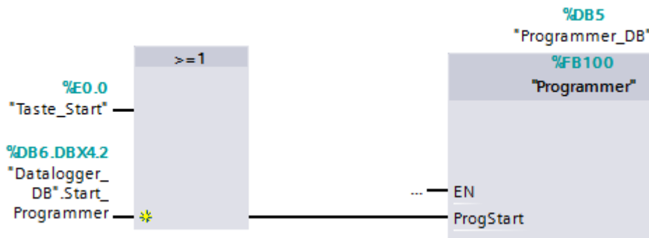
Programmer with wiring at ProgStart
